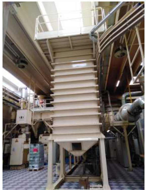
Single flat wall cell, smooth with exposed external stiffeners, on a metal structure, for raw coffee seeds.
